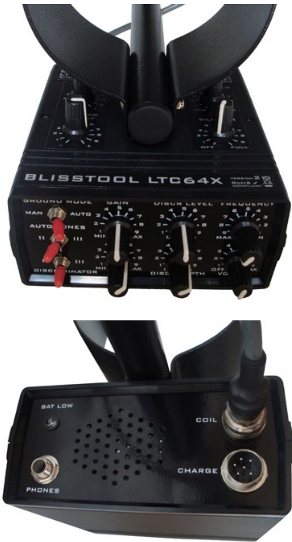
Fig.3 / Setting, indication and maintenance bodies of BLISSTOOL LTC64X
