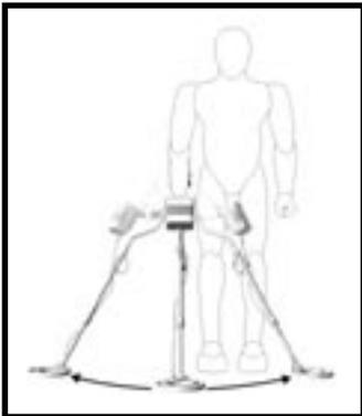
When the stem is properly adjusted, the 1212-X is balanced for sweeping in a tight semi-circle. Always overlap your sweeps at least 50%.
