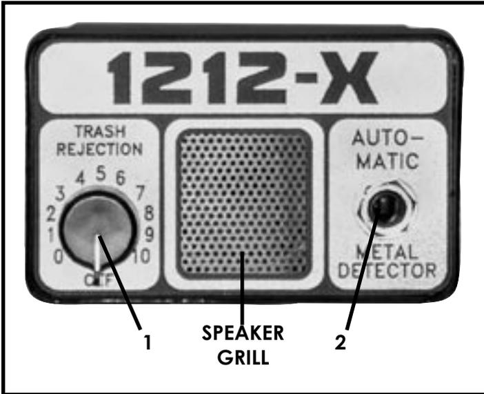
Figure 3. Control Panel. One knob does it all!
